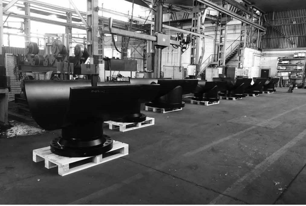
LS LineStop Fittingleri 600# RF 102 Bar (Madrid de bununan imalat atölyesinde)
